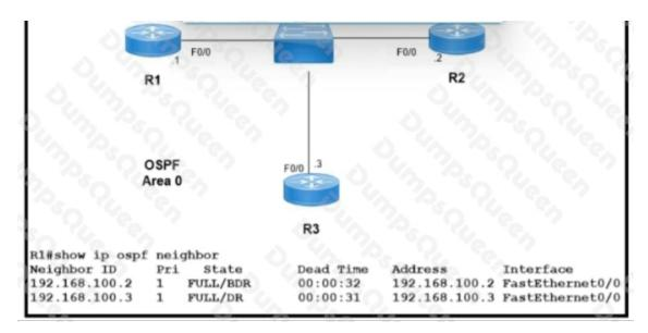
Which two configurations must the engineer apply on this network so that R1 becomes the DR? (Choose two.)
