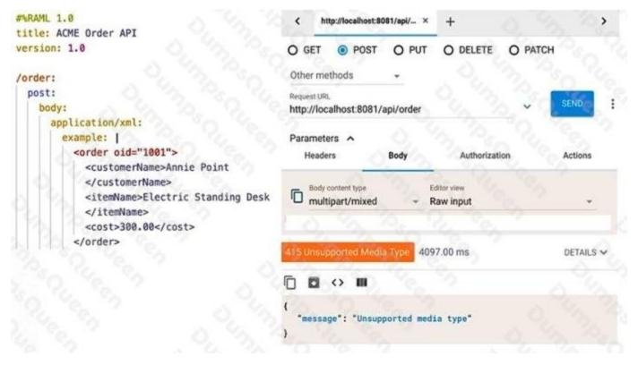
The web client sends a POST request to the ACME Order API with an XML payload. An error is returned.
